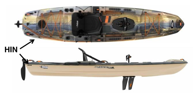
**HIN**: The hull identification number is a unique serial number comprised of 12 characters. It is located on the starboard (right) side of the hull, next to the stern.
